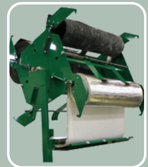
Optional Four Position Insulation Holder US Patent #7,926,757
